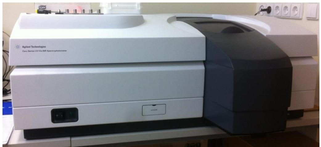
UV-Vis-mid-IR spectrometer Cary 5000 (Agilent)
