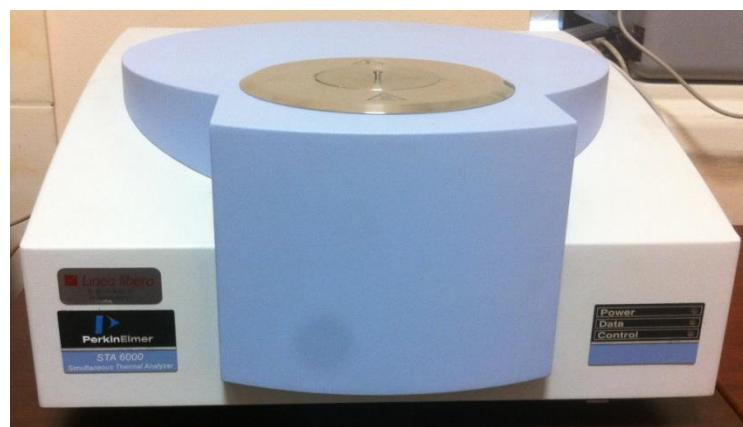
Simultaneous Thermal Analyzer STA 6000
